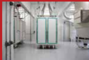
The latest 280 micron, four- section sifters from Buhler provide final sizing prior to loading.
